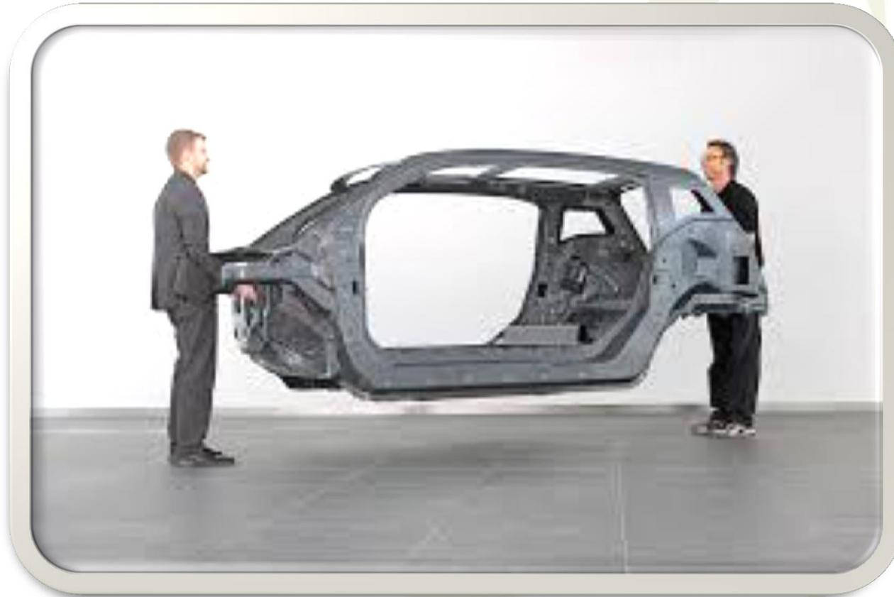
With the composite vehicle is expected to achieve a 20-25% reduction in vehicle weight and a 10-20% reduction in CO2 emissions
